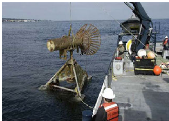
Figure 3.7. Recovering a docking system for an autonomous underwater vehicle after a test deployment in Monterey Bay. Photo by Brett Hobson ©2006 MBARI
