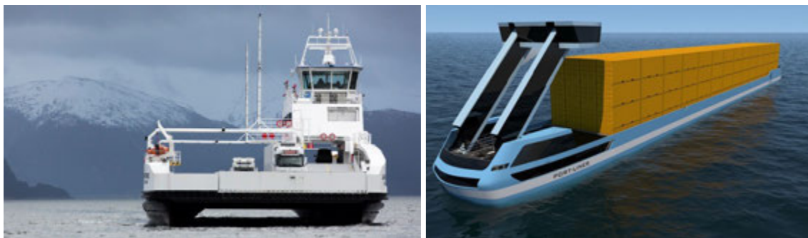
Figure 10.2. The first all-electric ferry operating in Norway, the MF Ampere (left) and the Port-Liner fully electric canal cargo vessel in development and capable of autonomous operation (right). Sources: www.siemens.com/press and Port-Liner
